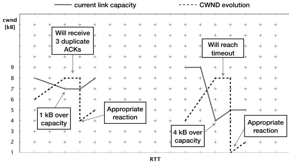
Reaction of the CWND (dashed line) if the current link capacity (continuous line) is exceeded by at most 2 kB (left) or by more than 2 kB (right).
