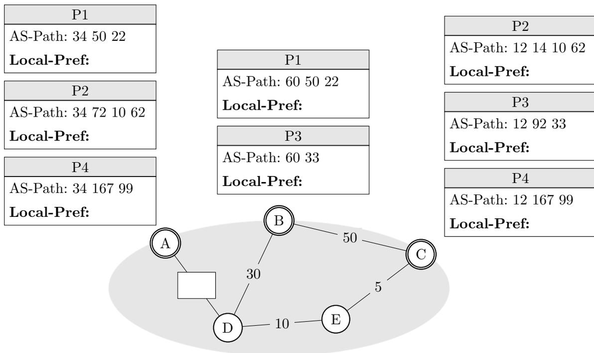
Figure 8: A simple BGP network forming an iBGP full-mesh.
