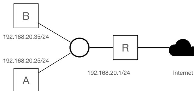
Figure 1: Two hosts connected through a router to the Internet.
