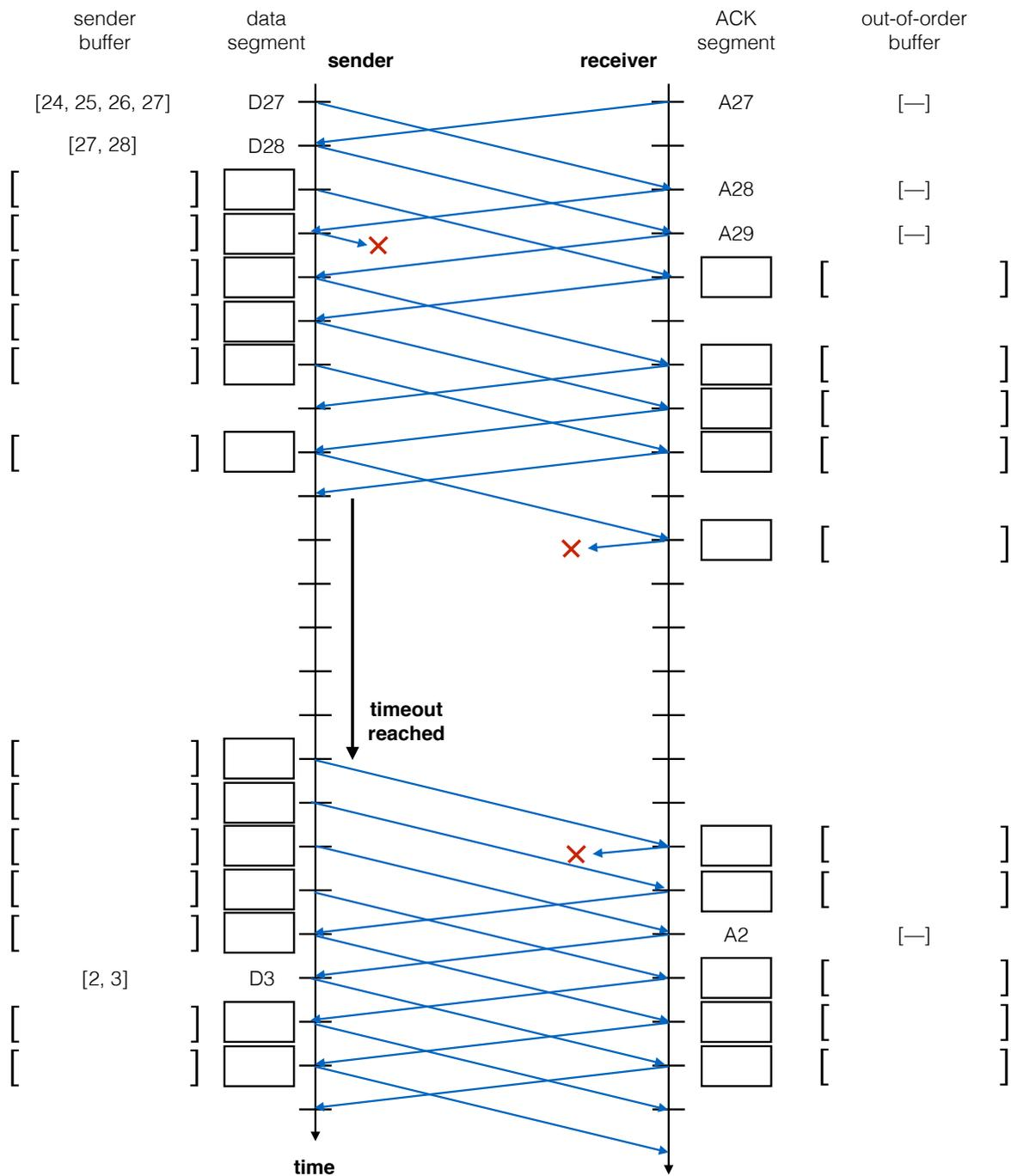
Figure 14: Incomplete time-sequence diagram of an ongoing connection using the previously described GBN protocol.
