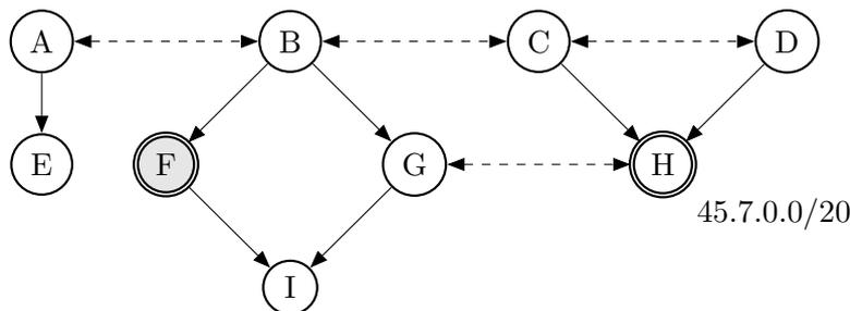
Figure 11: An Internet topology with 9 ASes. AS  $F$  aims at hijacking traffic destined to AS  $H$ .
