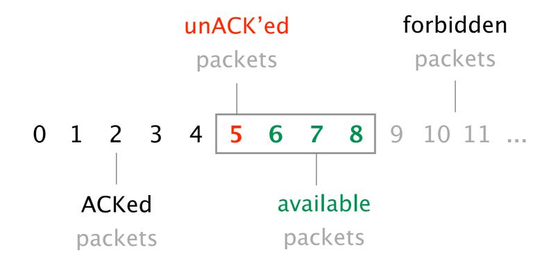
Timeliness of the window protocol depends on the size of the sending window Assuming infinite buffers,
