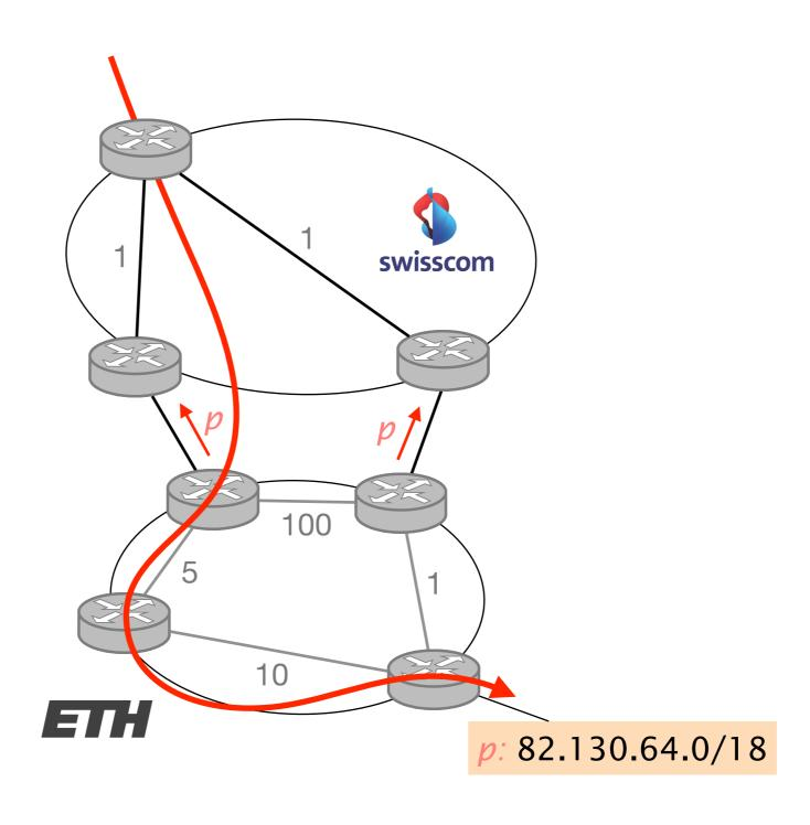
Yet, ETH would prefer to receive traffic for p on its right border router which is closer to the actual destination
