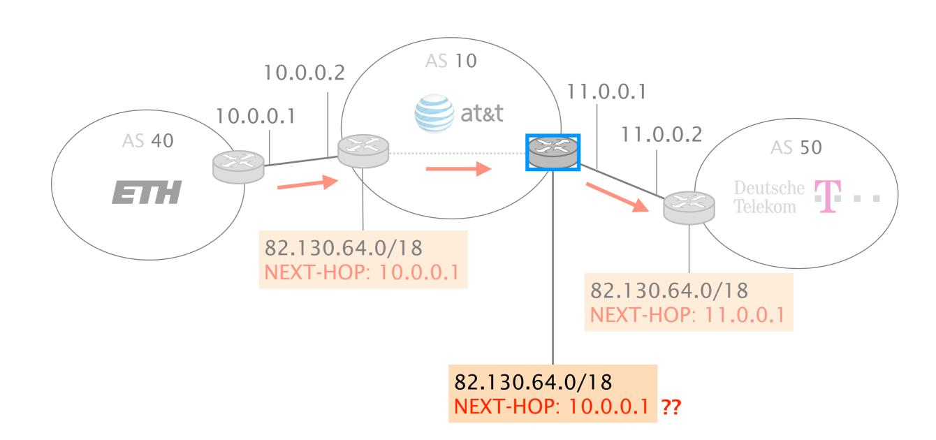
One solution is for the external router to redistribute the prefixes attached to the external interfaces into the IGP
