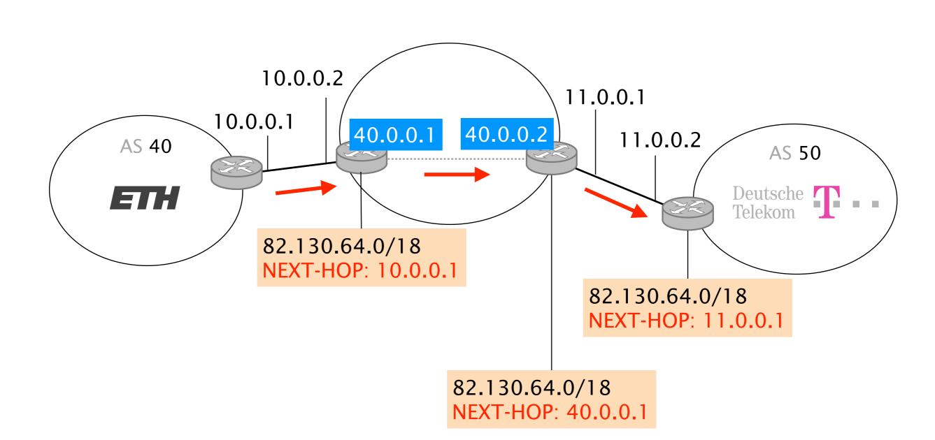
The advantage of next-hop-self is to spare the need to advertise each prefix attached to an external link in the IGP
