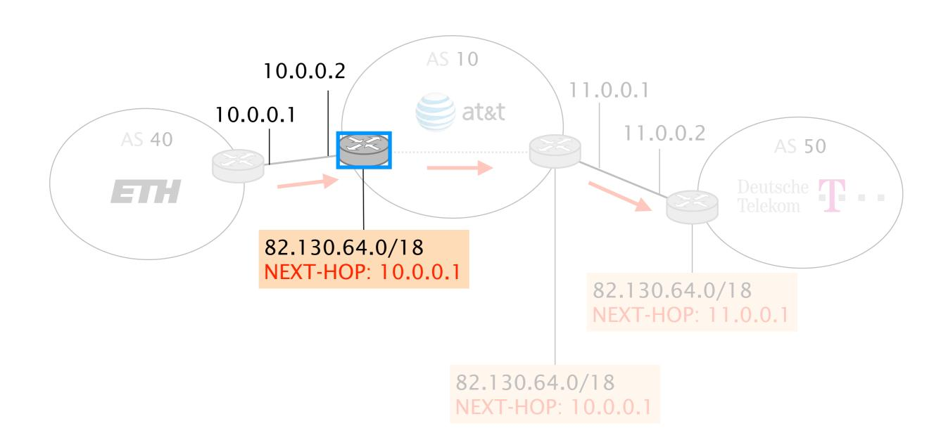
That router is *not* directly to the NEXT-HOP's subnet (10.0.0.0/30) and does not know how to reach it, it will therefore drop the BGP route...
