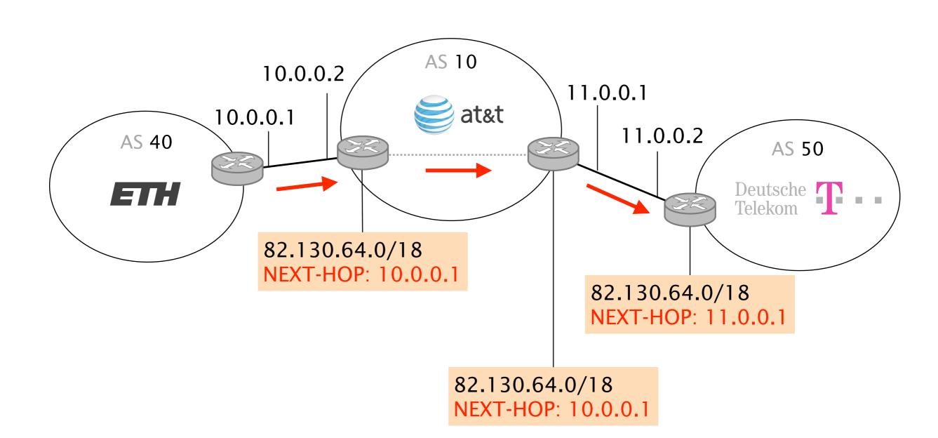
For externally-learned routes, this means that the NEXT-HOP is the IP address of the neighbor's eBGP router, here 10.0.0.1 for at&t
