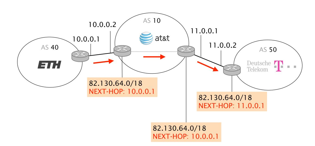
For this router, reaching 10.0.0.1 is not a problem as it is directly connected to the corresponding subnet (10.0.0.0/30)
