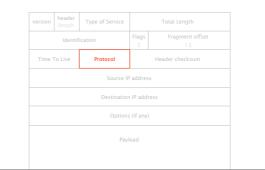
The checksum is the sum of all the 16 bits words in the header (does not protect the payload)
