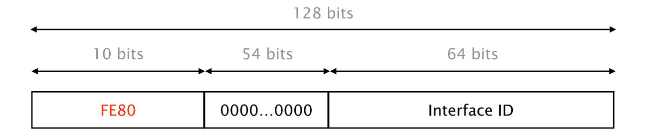
Each host/router **must** generate a link-local address for **each** of its interfaces
