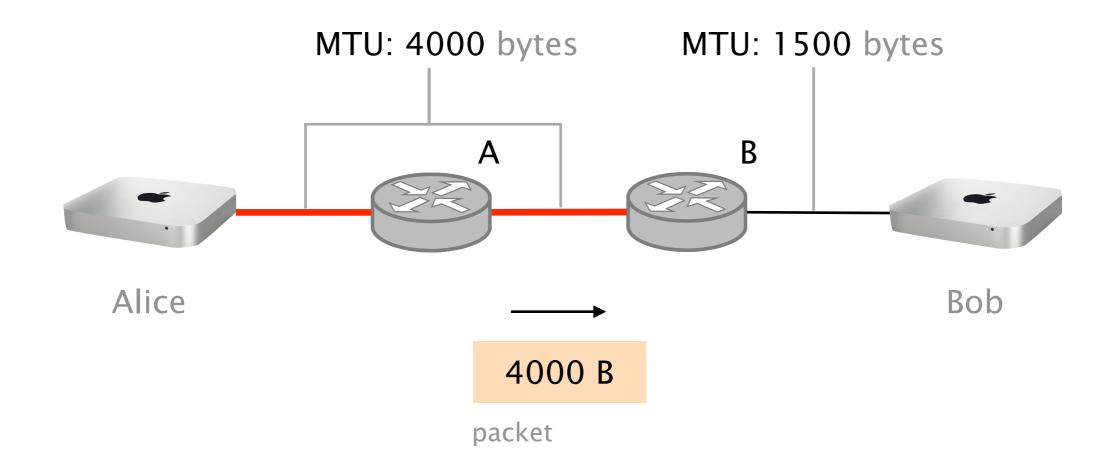
Because the packet is larger than the MTU, router B will split the packet into fragments
