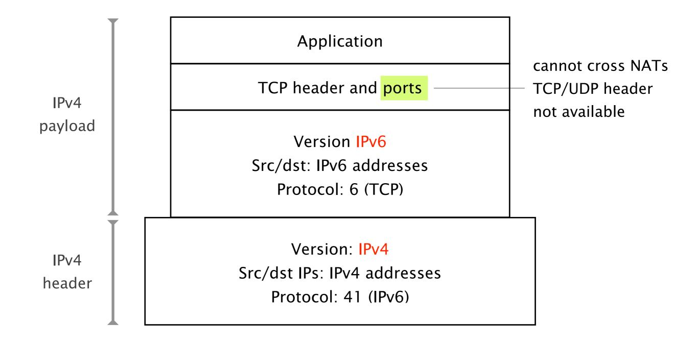
6to4 transmits IPv6 packets over IPv4 networks without explicit tunnels
