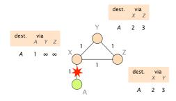
Consider the network on the left which uses distance vector routing with poisoned reverse. Each link is associated with a weight that represents the cost of using it to forward packets. Link weights are bi-directional.
