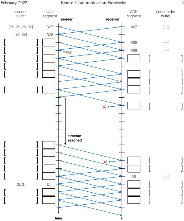
Figure 14: Incomplete time-sequence diagram of an ongoing connection using the previously described GBN protocol.
