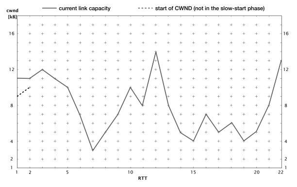
Figure 15: Copy of the CWND evolution in task 4 b) (iii).
