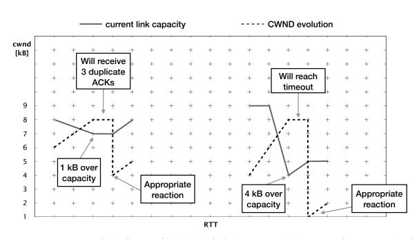
Figure 12: Reaction of the CWND (dashed line) if the current link capacity (continuous line) is exceed by at most 2 kB (left) or by more than 2 kB (right).
