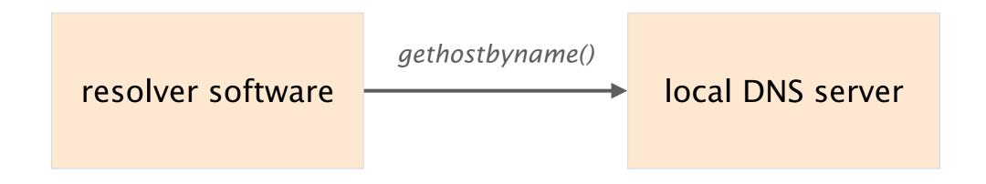
trigger resolution process send request to local DNS server usually, near the endhosts
