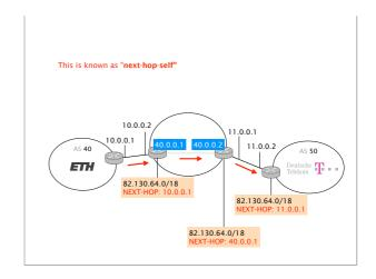
The advantage of next-hop-self is to spare the need to advertise each prefix attached to an external link in the IGP
