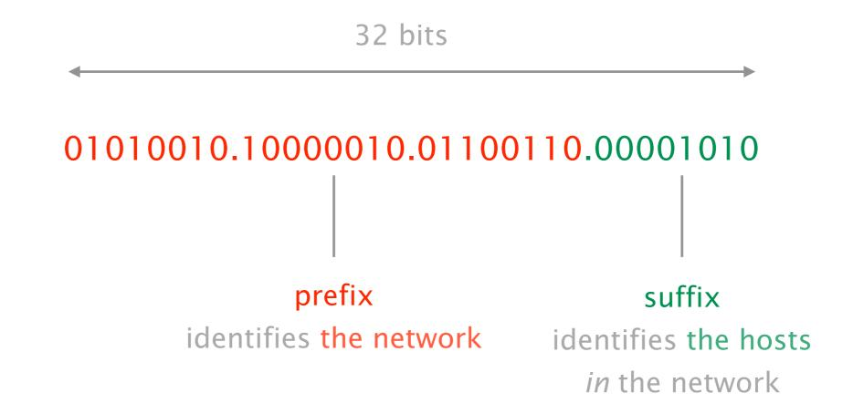
Routers forward packet to their destination according to the network part, *not* the host part
