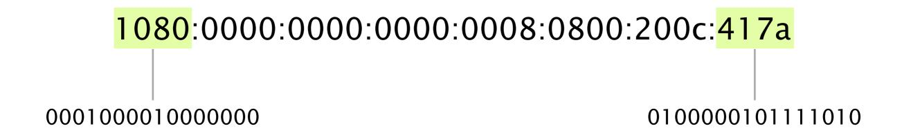
IP addressing is hierarchical, composed of a prefix (network address) and a suffix (host address)
