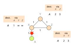
Consider the network on the left which uses distance vector routing with poisoned reverse. Each link is associated with a weight that represents the cost of using it to forward packets. Link weights are bi-directional.
