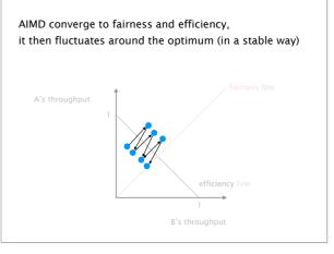
AIMD converge to fairness and efficiency, it then fluctuates around the optimum (in a stable way)
