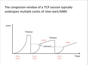
TCP congestion control in less than 10 lines of code Initially: cwnd = 1 ssthresh = infinite New ACK received: if (cwnd < ssthresh):
