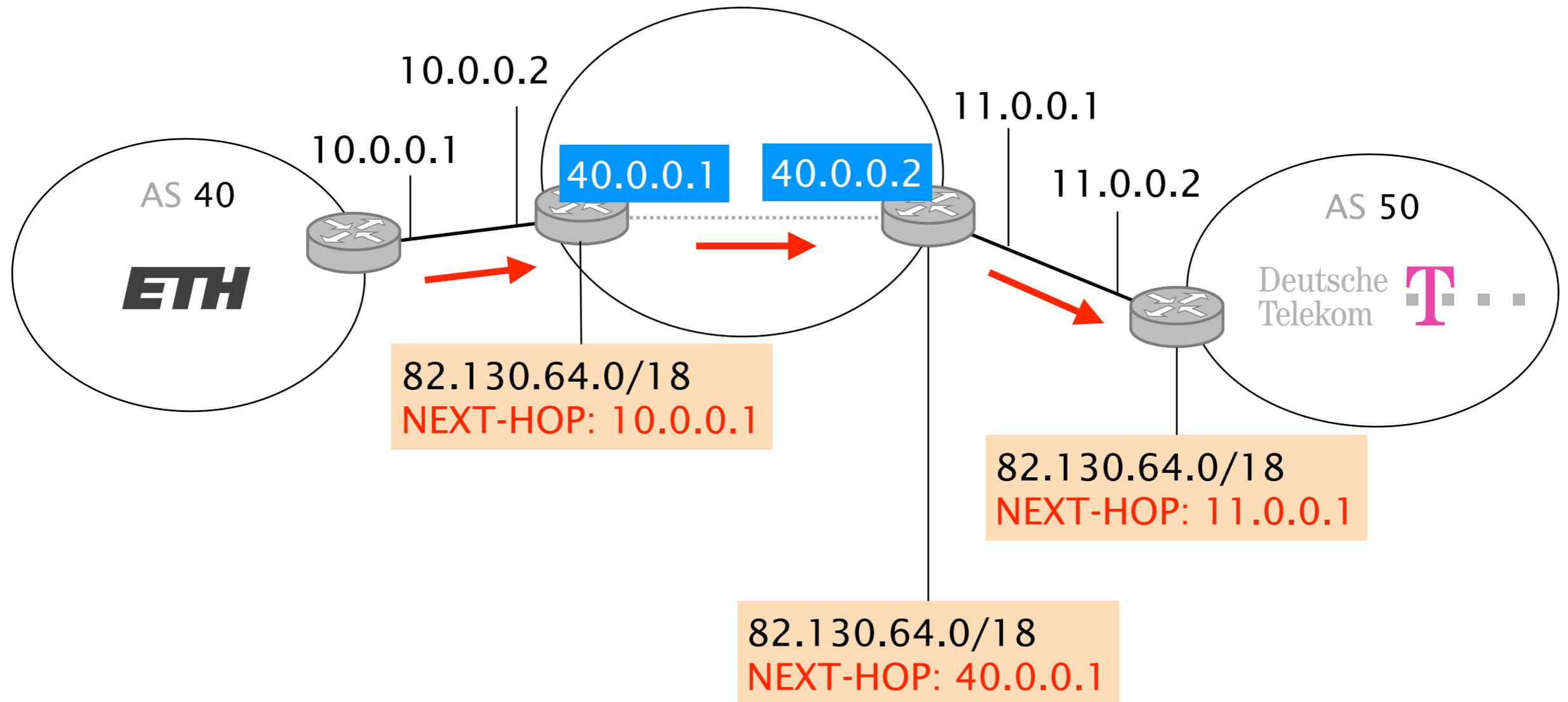
The advantage of next-hop self is to spare the need to advertise *each* prefix attached to an external link in the IGP
