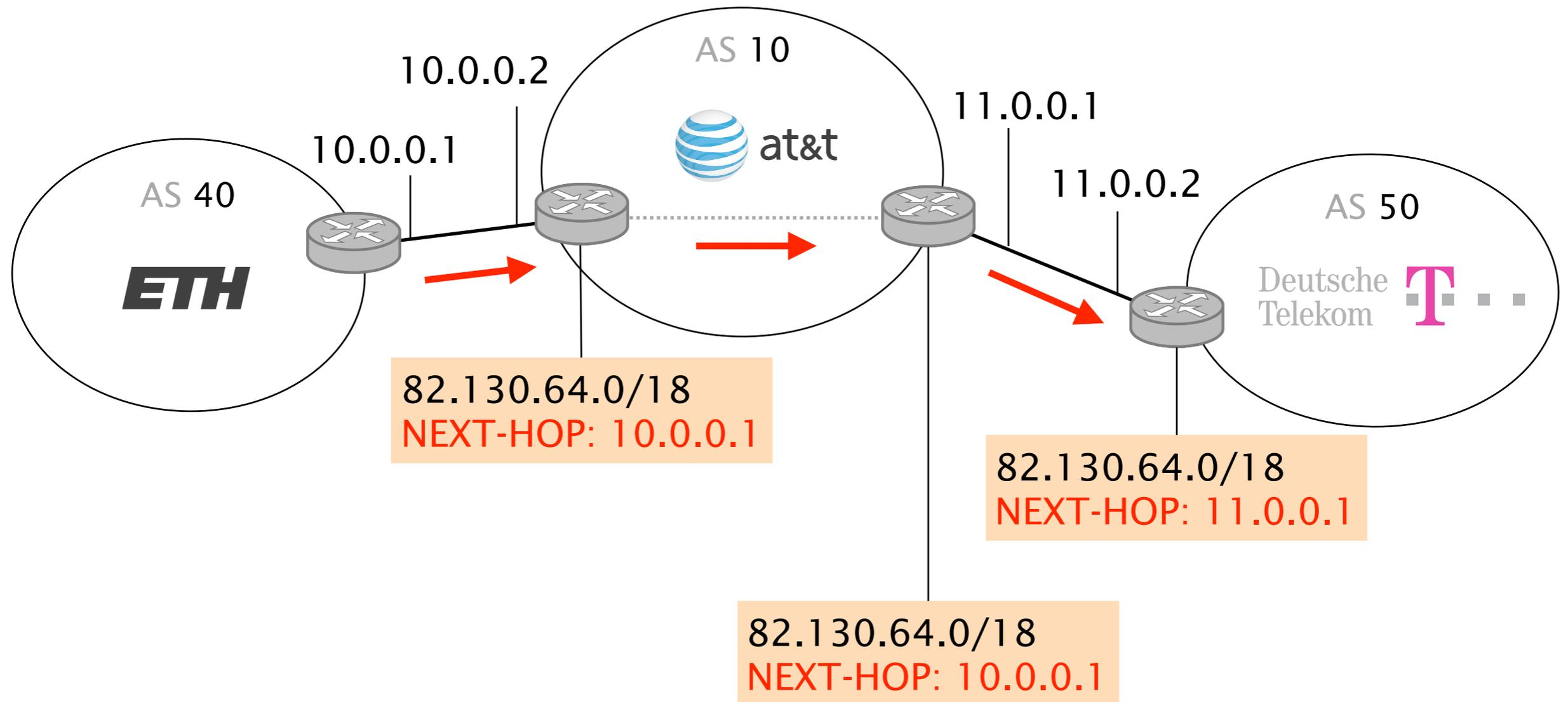
For externally-learned route, this means that the NEXT-HOP is the IP address of the neighbor's eBGP router, here **10.0.0.1**
