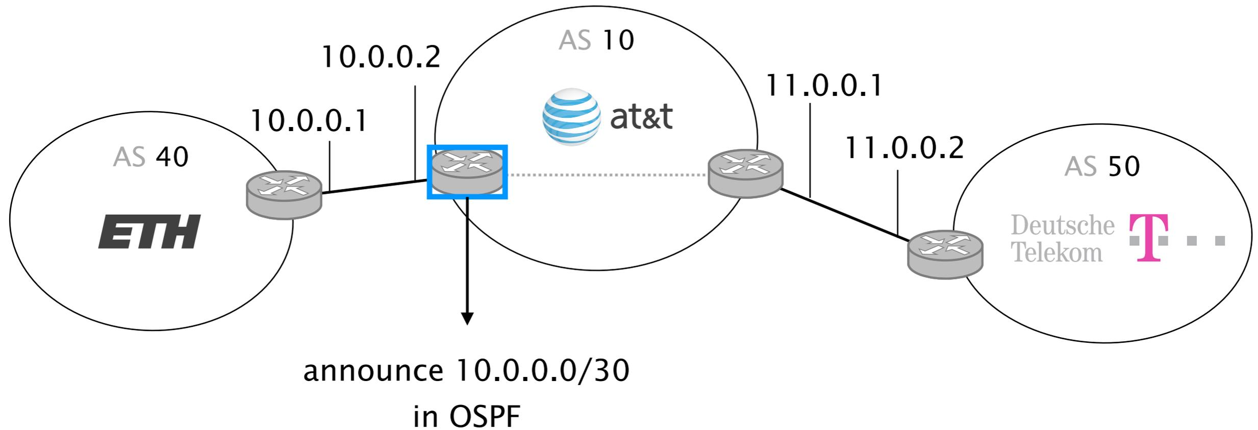
Another solution is for the border router to rewrite the NEXT-HOP before sending it over iBGP, usually to its **loopback address**
