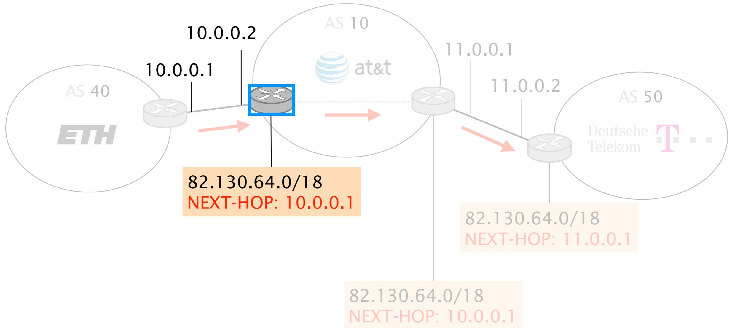
That router is *not* directly to the NEXT-HOP subnet (10.0.0.0/30) and does not know how to reach it, it will therefore drop the BGP route...
