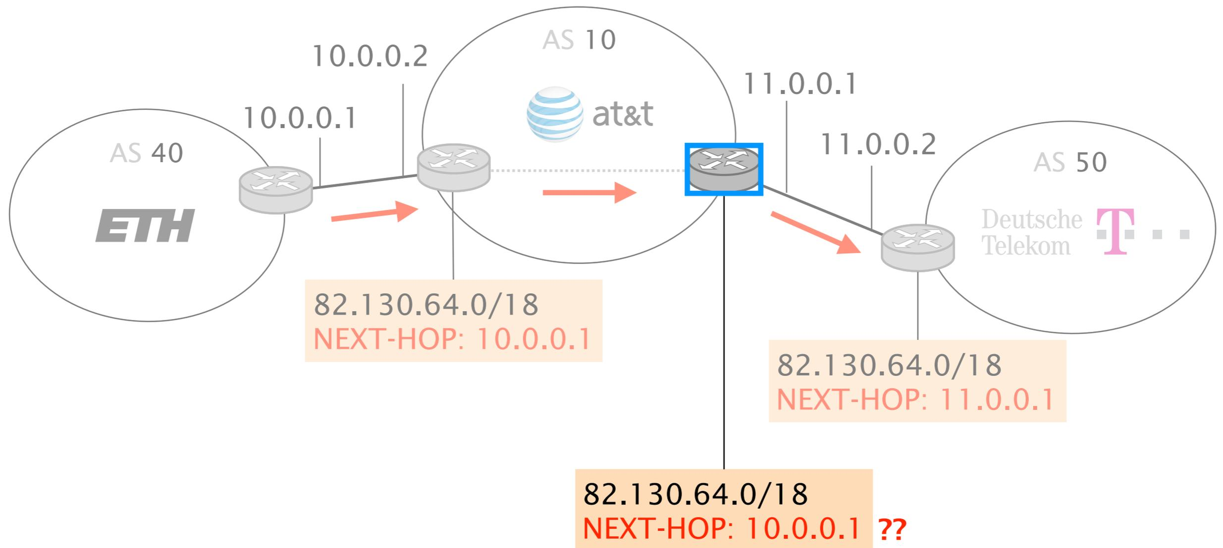
One solution is for the external router to redistribute the prefixes attached to the external interfaces into the IGP
