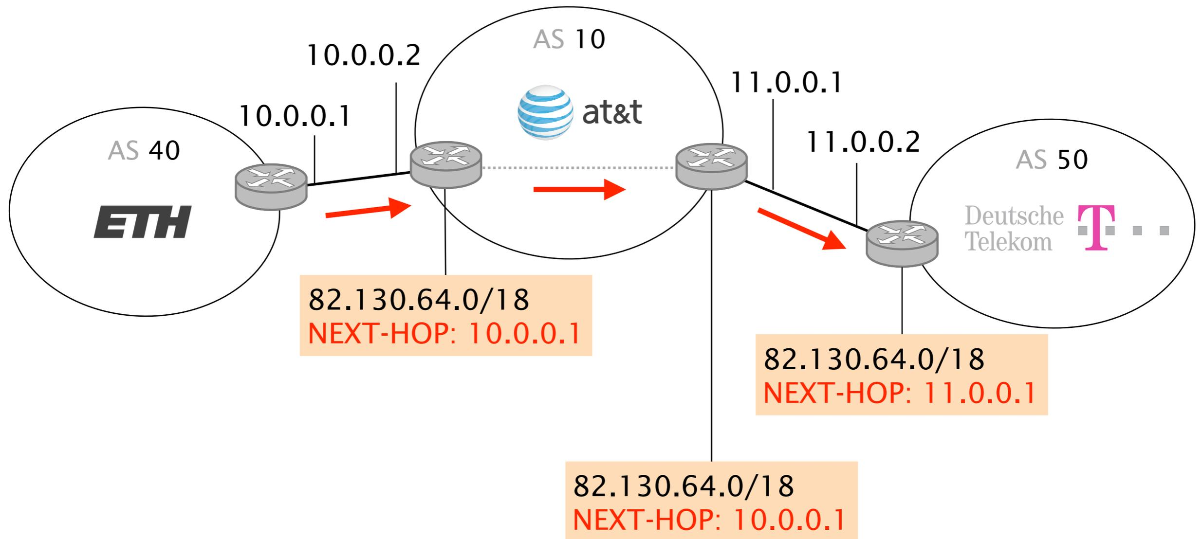
For this router, reaching 10.0.0.1 is not a problem as it is directly connected to the corresponding subnet (10.0.0.0/30)
