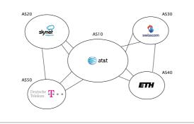
Using BGP, ASes exchange information about the IP prefixes they can reach, directly or indirectly
