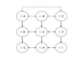
Tier-1s must be connected through a full-mesh of peer links
