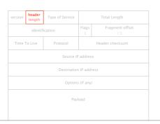
The ToS allows different packets to be treated differently, e.g., low delay for voice, high bandwidth for video
