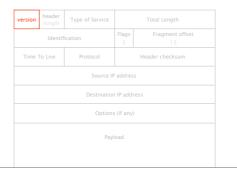
The header length denotes the number of 32-bits word in the header, typically set to 5 (20 bytes header)
