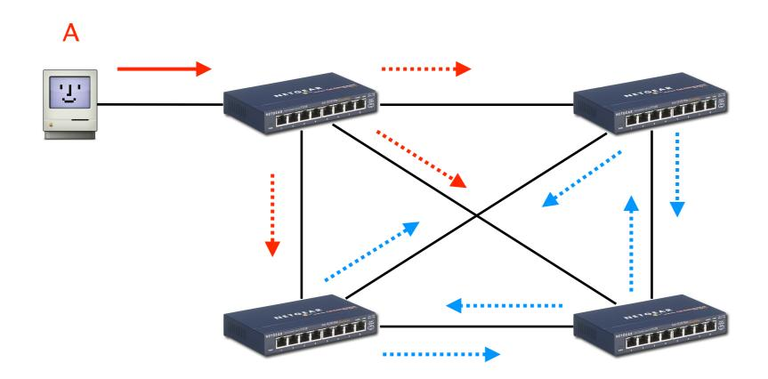
Each frame leads to the creation of *at least two new frames!* exponential increase, with no TTL to remove looping frames...
