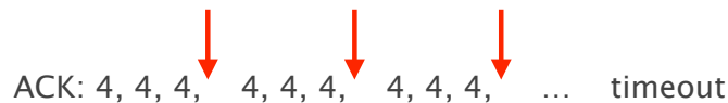
Figure 4: At each red arrow the sender should re-send (Selective Repeat) data segment 4.
