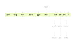
The bottom (and bulk) of the hierarchy is managed by Internet Service Provider or locally
