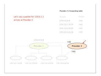
When a router receives an IP packet, it performs an IP lookup to find the matching prefix
