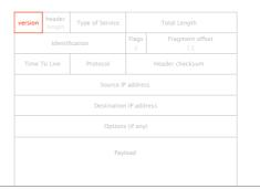
The header length denotes the number of 32-bits word in the header, typically set to 5 (20 bytes header)
