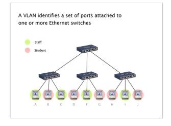
Switches need configuration tables telling them which VLANs are accessible via which interfaces
