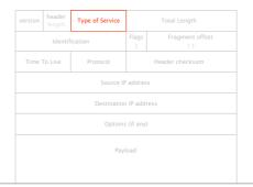
The total length denotes the # of bytes in the entire packet, with a maximum of 65 535 bytes
