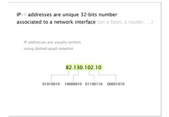
Routers forwards IP packets based on their destination IP address
