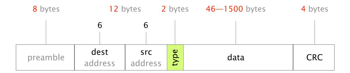
Ethernet efficiency (payload/tot. frame size): ~97.5%
