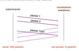
To solve this issue, we need a mechanism for flow control
