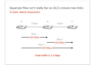
With equal-per-flow, A ends up with 1 Gbps because it sends 2 flows, while B ends up with 500 Mbps
