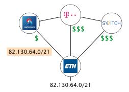
ETH is connected to three providers with different costs.
