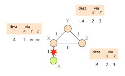
Consider the network on the left which uses distance vector routing with poisoned reverse. Each link is associated with a weight that represents the cost of using it to forward packets. Link weights are bi-directional.
