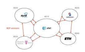
Using BGP, ASes exchange information about the IP prefixes they can reach, directly or indirectly
