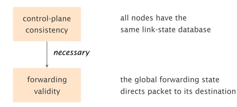
Inconsistencies lead to transient disruptions in the form of blackholes or forwarding loops Blackholes appear due to detection delay, as nodes do not immediately detect failure
