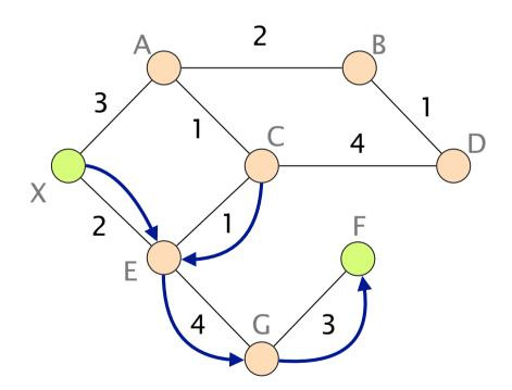
The loop disappears as soon as E updates its forwarding table Convergence is the process during which the routers seek to actively regain a consistent view of the network
