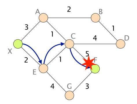
C learns about the failure and immediately reroute to E
