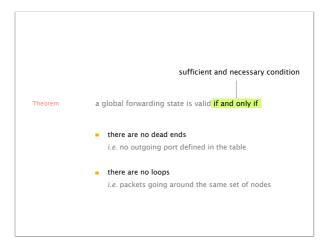
No dead ends and no loops are a sufficient and necessary condition for forwarding validity
